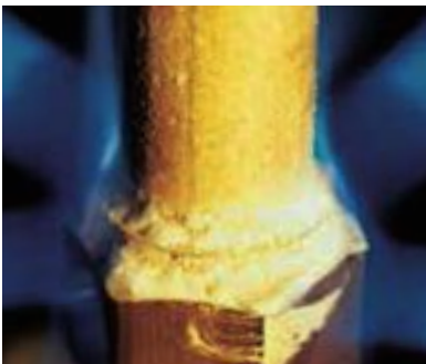
The flux becomes white and solidifies as water is driven off
